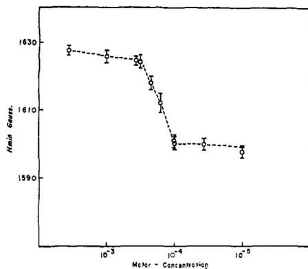
Figure 3. Variation of  $H_{\min}$  with concentration of thiopyronine in ethanol at 77°K and a microwave frequency of 9239 MHz.
