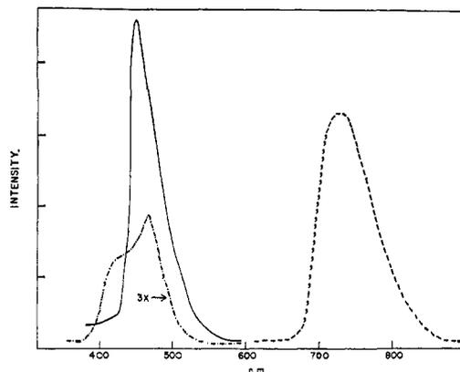
Figure 2. Phosphorescence spectra at 77°K of —, thioxanthene; ---, thiopyronine; and ·····, thiopyronine in ethanol at a concentration of  $10^{-3}$  M.
