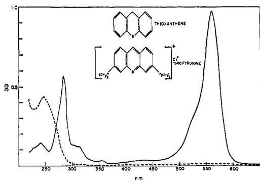
Figure 1. Absorption spectra: ---,  $10^{-5}$  M thioxanthene; —,  $10^{-5}$  M thiopyronine in ethanol.
